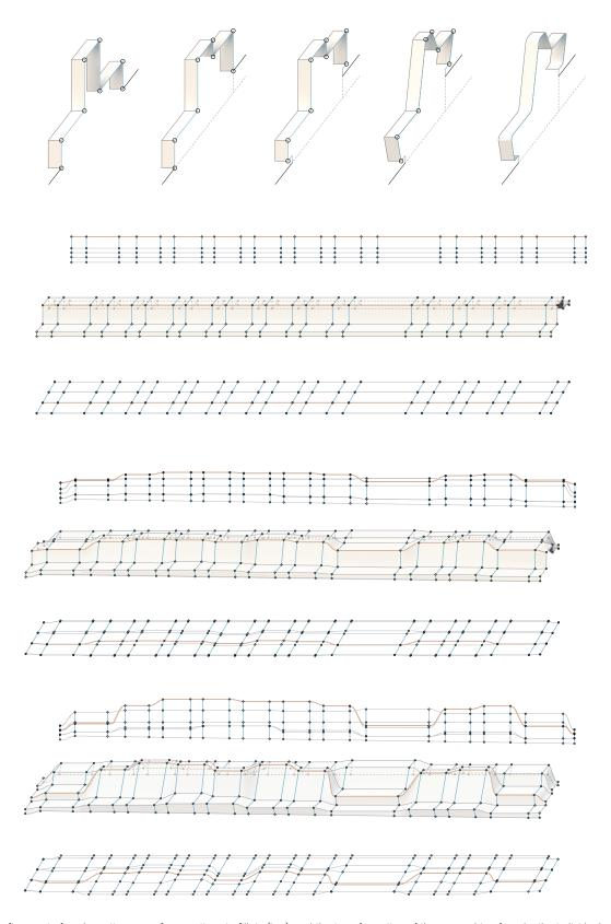
The gradual refinement of each section curve from vertices to fillets (top), and the transformation of the overarching form by the individual control through control curves in plan and section (three iterative steps of transformation). Comparison generated model and final bench (right page).
