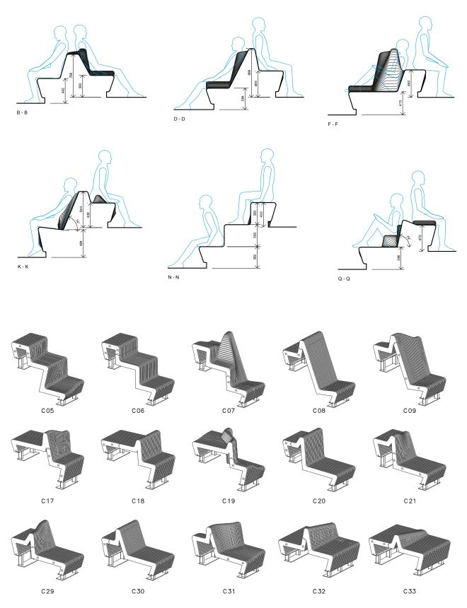
Examples of representations used throughout the design process - cross sections with scale figure to assess bench proportions and comofort (top), and ezonometric views of selected modules (bottom). Snapshots from auto-generated dimensioning tool (right page).
